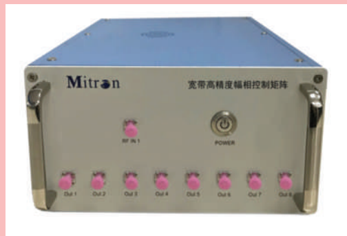
▲ Fig. 2 Block diagram of a 1x8-way phase and amplitude control matrix (a). The size of the unit is 220 mm x 290 mm x 150 mm (b).
