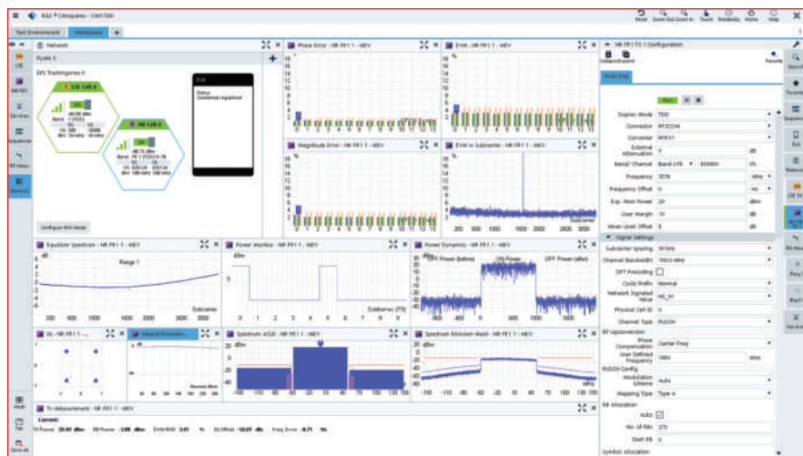
Fig. 2 The test software R&S CMSquares controls all 5G radio communications testers, unifying 5G NR testing.
